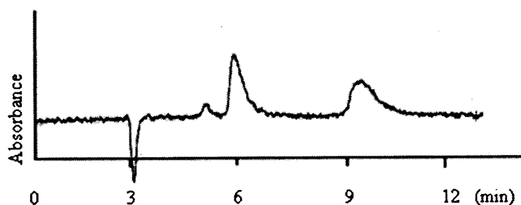
Figure 4.2. Enantioseparation of CB-cyclam 1mg/mL Mobile Phase: 15/85/2 (v/v/wt %) ethanol/hexane/diethanolamine Flow rate: 1.0 mL/min Column: Chiralpak AD (250 × 4.6 mm; 10 \mu m) Detection \lambda : 237 nm Temperature: 23 °C Injection: 10 \mu L of 1 mg/mL CB-cyclam
